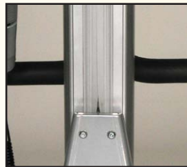
Mast shroud protects lifting chain
