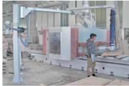
Articulated-arm jib to move around obstacles
