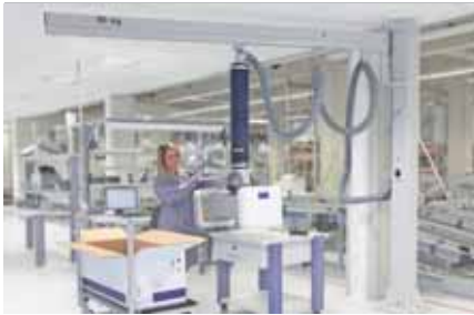
Flat jib for particularly low ceilings
