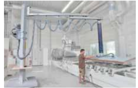
Telescopic jib for confined working areas
